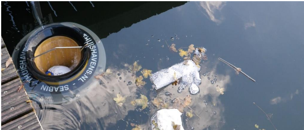
Kuva 27. Seabin meriroskakori (Seabin, https://seabinproject.com/the-seabin-v5/ )
